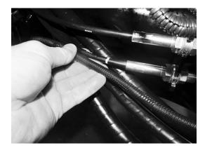
3.6.7 Follow the existing Harness Assembly, Third Function (20) up to the SCV wire as shown in the illustration.
