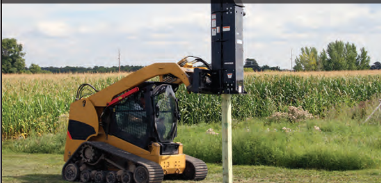
Manually adjusted speed to control blows per minute up to 40 bpm
