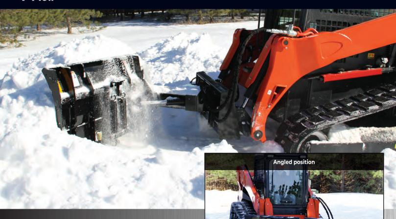
The V-Plow has a 10 gauge steel body with 5/16" plate ribs on the back that run the full length making for an extremely rigid and strong backbone.
