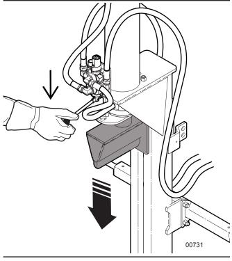
Fig. 5-Extend Wedge to split Wood
