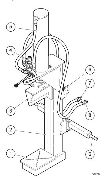
Fig. 3-WX350, WX360 Wood Splitter Components
