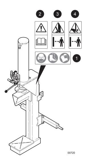
Fig. 2-Safety Decal Locations (typical for WX350, WX360 models)
