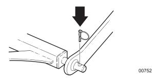
Fig. 10 - Attach Lift Arms and Lynch Pins
