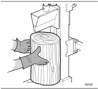
Fig. 13-Correct Log Placement
