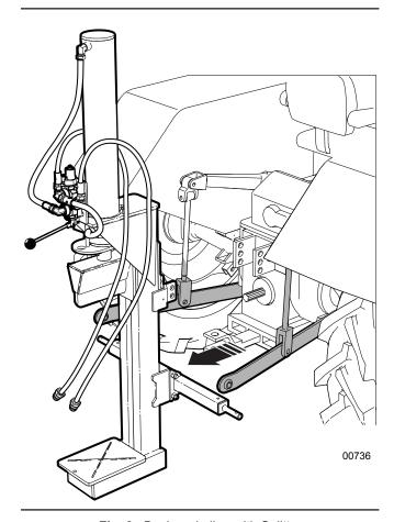
Fig. 9-Back-up in line with Splitter
