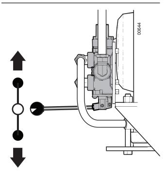
Fig. 4-Splitter Control Valve
