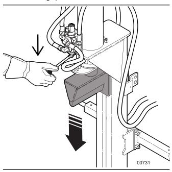
Fig. 14-Extend Wedge to split Wood
