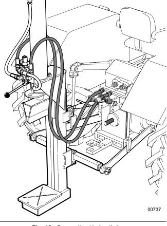
Fig. 12-Connecting Hydraulic hoses
