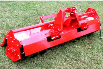
The reverse rotation of our tiller tines forces the tiller down into the ground for deep smooth cultivation while bringing debris up over the top of the rotor. This unique action deposites larger debris first then covers it with finely pulverized soil particles for a
