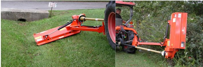
Available in working widths of 47 inches, 60 inches, and 75 inches The hydraulic system enables you to use the tool behind the tractor or alongside the tractor. Used for ditch banks and hill sides Standard Features Include:
