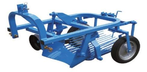
CPP-T Potato Harvestors feature a hardened vibrating digging plowshare with adjustable digging depth that conveys the potatoes and soil onto a vibrating sieve grid. This separates the potatoes from the soil and deposits them in an easy to access single cut row.
