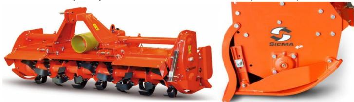
The T25 Series Heavy Duty Gear Drive Tillers feature an easy change 4 speed gearbox allowing you to set your tiller speed to match field conditions. The load bearing frame on which the gearbox and super heavy duty protective hood are mounted make this machine extremely sturdy for even the most demanding applications. All Phoenix line tillers are specially designed to reduce the possibility of clogging even in wet or sticky soil conditions.
