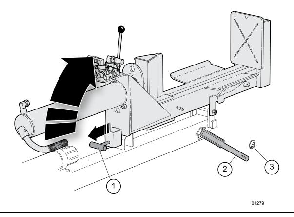
Fig. 10-Rotate Splitter to Vertical
