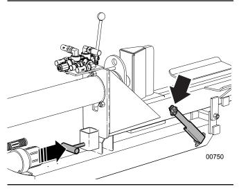
Fig. 17-Lock Pin and Latch Engaged
