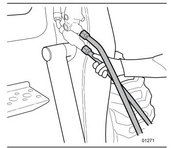
Fig. 11 – Connect pressure and return hoses
