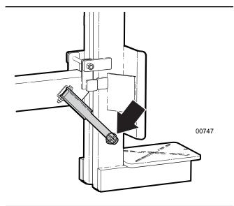
Fig. 9-Locking Latch in Place
