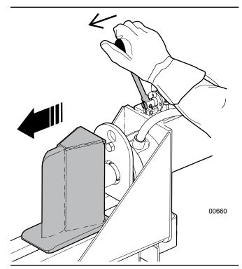
Fig. 5-Extend Wedge to split Wood
