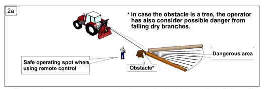
• The winch operator must constantly observe the load being pulled. If the pulling distance is not visible from his position, an assistant being in constant contact with the operator must observe the load. The winch operator and assistant communicate with previously agreed signs (Figure: 2b).
