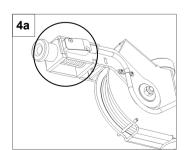
**Limit switch (Fig. 4a)** automatically shuts down pulling, when rope is fully coiled.
