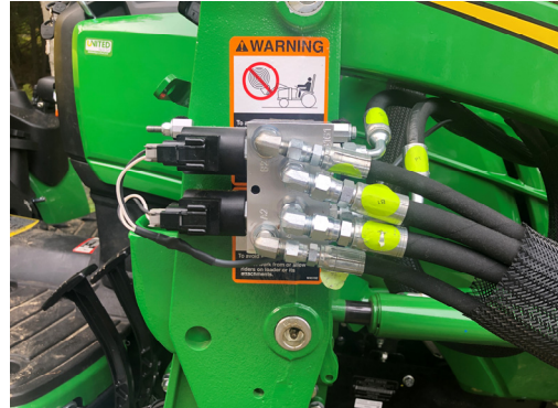
Fig. 1 (Diverter Valve Location)
