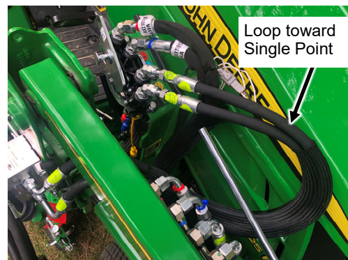
Fig. 3 (Loop Gang of 2 Hoses toward Single Point)
