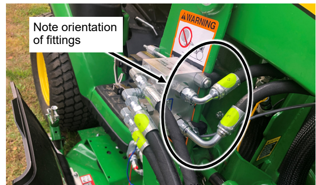
Fig. 2 (Attach Gang of 2 Hoses to Valve)
