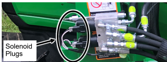
Fig. 5 (Attach Wire Harness Plugs to Solenoids)
