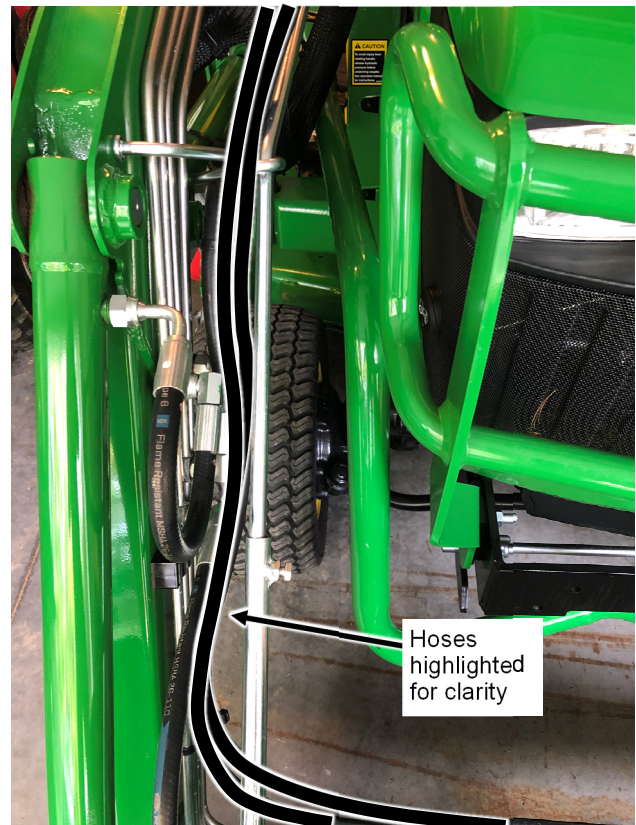
Fig. 3 (Route Gang of 4 Hoses up Loader)
