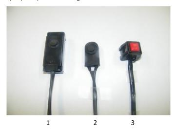
Attach configuration 1 to the joystick using two cable ties thru the provided openings near the ends of the plastic housing (see below left). If your joystick has a bend close to the knob, such that the plastic switch housing will not fit, depress the 4 tabs on the plastic housing to open it, exposing the rubber switch inside. Discard the plastic housing and mount the rubber switch (configuration 2) with two cable ties located close together as shown below and to the right.
