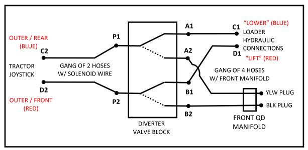
Refer to the image above for an overall understanding of the hydraulic connections.
