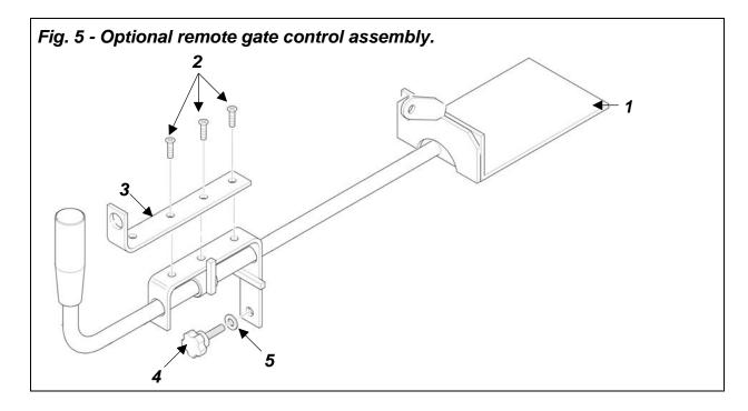
To assemble the remote gate control on the spreaders proceed as follows (see fig. 5):
