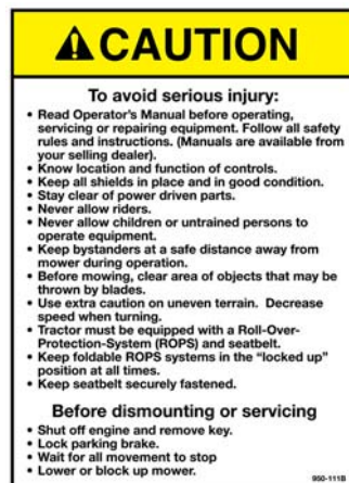
Fig. 2 - Safety decals - implement; replace immediately if damaged.
