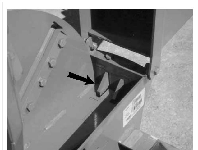
View of twig breaker teeth inside rotor compartment
