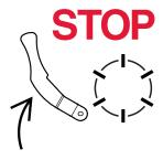
IMPORTANT! Be aware once the rotor is disengaged, the clutch brake automatically engages.
