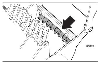
Fig. 43-Chop Block in Rotor Housing
