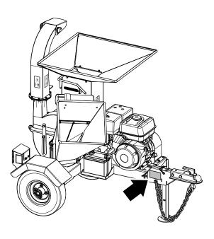
Fig. 1-Serial Number Plate Location
