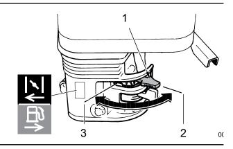
Fig. 20-Choke Lever
