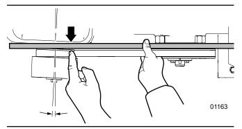
Fig. 36-Engine Mount Misalignment
