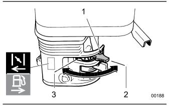
Fig. 8-Choke Lever
