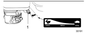
Fig. 21 - Engine Throttle
