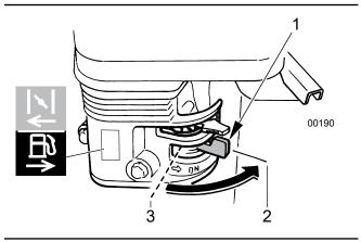
Fig. 9-Fuel Valve Lever
