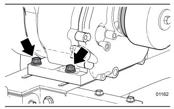
Fig. 37 - Engine Mount Bolts
