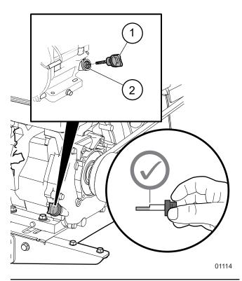
Fig. 18-Engine Oil Level check
