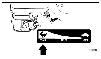
Fig. 23-Move throttle setting to MAX
