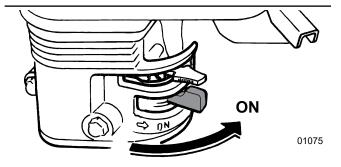
Fig. 19-Fuel valve Lever
