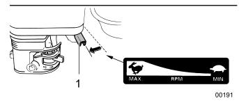
Fig. 10 - Throttle Lever Positions
