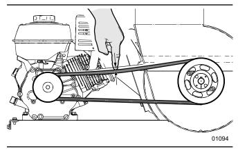
Fig. 34-Rotor drive belt tension
