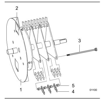
Fig. 44 - Rotor Assembly
