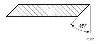
Fig. 40 - Sharpen Blade at 45° angle
