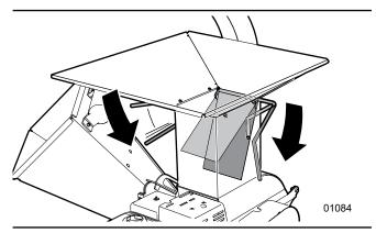
Fig. 12-Feed Gate Levers
