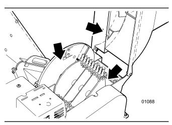
Fig. 30 - Clear out areas inside of chipper
