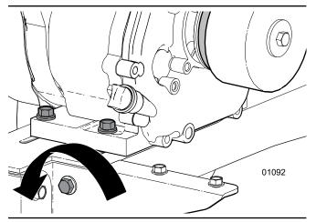
Fig. 33 - Drive Belt Tension Adjuster Bolt
