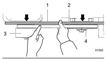
Fig. 35-Drive Belt alignment
