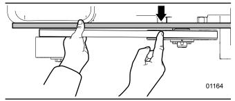
Fig. 38-Rotor Sheave Misalignment
