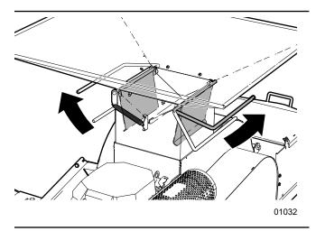
Fig. 7-Feed Gate Levers
