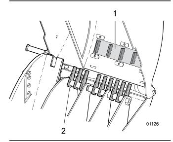
Fig. 36-Chop Block in Rotor Housing
