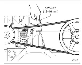
Fig. 23-Rotor drive belt tension
