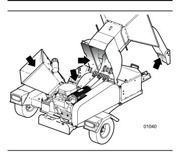
Fig. 18 - Clear out areas inside of chipper
