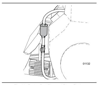
Fig. 39-Engine Fuel Filter and Shut-off Valve
