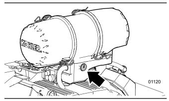
Fig. 20 - BXMT4238 Air Filter Restriction indicator
