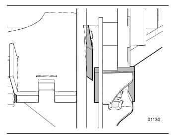
Fig. 33 - Checking ledger knife clearance
