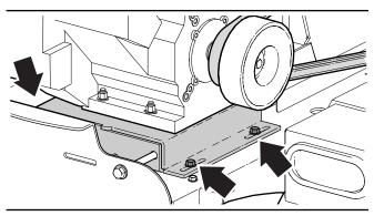
Fig. 27 - Engine Mount Bolts
