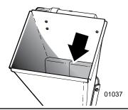
Fig. 15-Feed Hopper Safety Curtain
