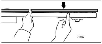
Fig. 28 - Rotor Sheave Misalignment
