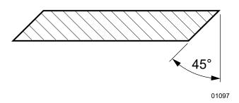
Fig. 30 - Sharpen Blade at 45° angle
