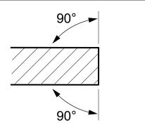
Fig. 35-Sharpening Ledger Knife
