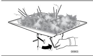
Fig. 16-Shredder Feed Control Handles
