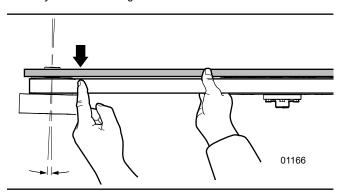
Fig. 25-Engine Mount Misalignment
