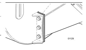
Fig. 32-Ledger knife inside lower rotor housing
