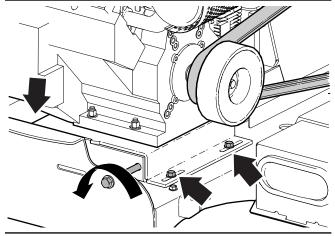
Fig. 22-Drive Belt Tension Adjuster Bolt
