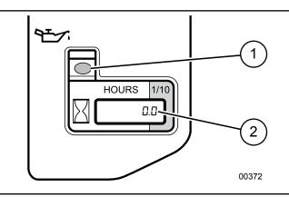
Fig. 9-Engine Hours and Oil Level Alert
