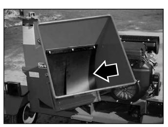
Fig. 16-Safety Curtain inside Feed Hopper
