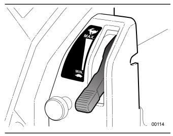
Fig. 6-Throttle Lever
