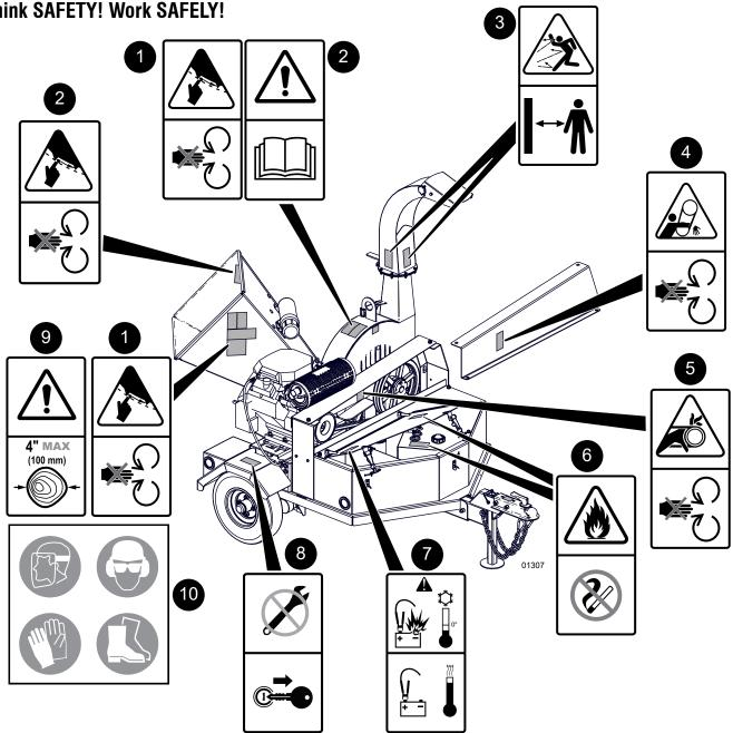
Fig. 2-Safety Signs on the machine
