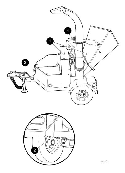
Fig. 22-Grease Points (typical of all models)
