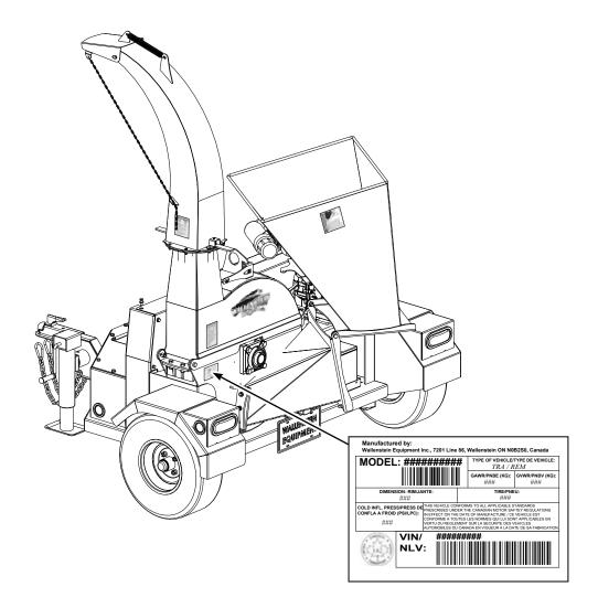
Fig. 1-Serial Number Location (typical)
