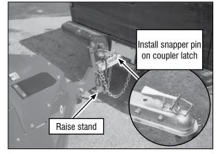
Fig. 12-PIN / STAND / SAFETY CHAIN / WIRING HARNESS
