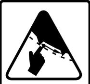
**Never reach into the feed hopper when the chipper is operating. Doing so risks contacting knives on the rotor and causing serious injury.**
