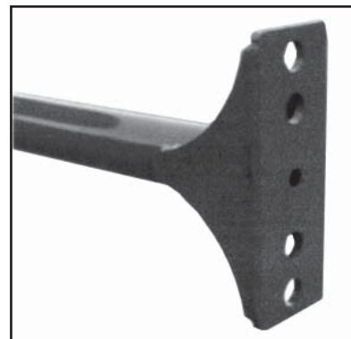
Tow-Bar Height Adjustment Slots
