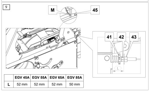
During the operation and under the load, the drive chain stretches, therefore the operator must check and readjust the chain periodically to prevent excessive wear of the whole chain drive. The chain must not be set to tight and chain slack should be set 1 to 3 mm. Shorther chain should allow  $\pm 1$  mm slack and longer chain  $\pm 3$  mm. Check the tightness of the chain by hand, pushing the chain between the chain wheels.
