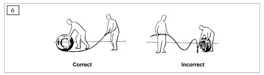
The wire rope release power must be set correctly, so the drum stops immediately after releasing the wire rope. This prevents the wire rope on the drum from releasing by itself.
