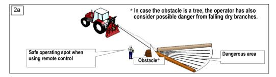
• The winch operator must constantly observe the load being pulled. If the pulling distance is not visible from his position, an assistant in constant contact with the operator must observe the load. The winch operator and assistant communicate with previously agreed signs (Figure: 2b).
