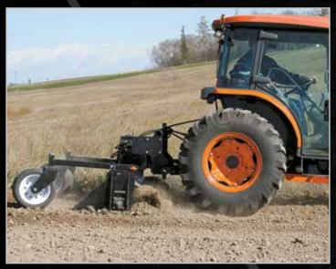
The aggressive teeth on the large-diameter rotor pulverize soil like an ordinary tiller, with the benefit of faster ground speed.
