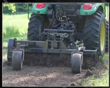
The 3-Point Soil Conditioner separates rocks, tears up sod, and pulverizes dirt clods.
