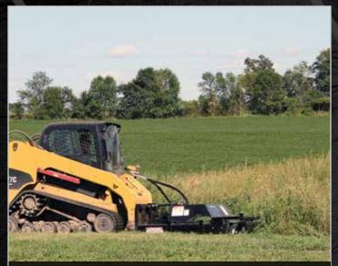
Two heavy-duty stump jumpers designed to store rotational energy.
