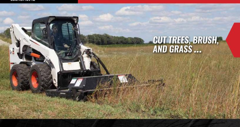
The Dual Rotary Brush Mower is engineered for today's larger skid steers. The 84" cutting width is built with 1/4" steel to withstand the rigors of brush cutting. Use it to cut trees, brush, and unwanted weeds and grass. It's unique automatic Float-n-Tilt™ system allows you to cut evenly on level surfaces as well as the most rugged terrain. This is further supported by the innovative blade positioning that achieves reduced deck length.
