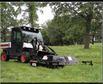
Closed front deck keeps material under the deck longer for finer mulching and to help prevent flying debris.
