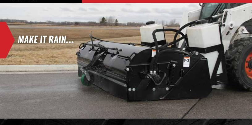
The Dust Control Water Kit is crucial for environments where dust suppression is a must. Compatible with our Power Angle Broom and Pick-Up Broom, as well as third party broom attachments, this unit mounts between the attachment and the skid loader. Light user assembly required for hoses and fittings.
