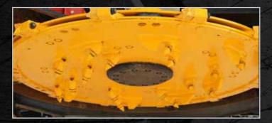
Tooth Protector Fins are made of hardened <sup>3</sup>/4" AR400 to protect the outer 8 teeth from direct impact with rocks and other debris.
