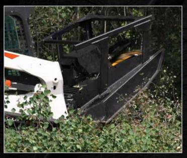
Clean deck design reduces amount of debris buildup, is easy to clean off and creates excellent visibility of the front work area.
