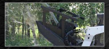
Unique slanted push bar prevents unwanted trees from hanging on the deck after cutting. This boosts productivity and safety by keeping the operator in the cab and not outside pulling branches off.
