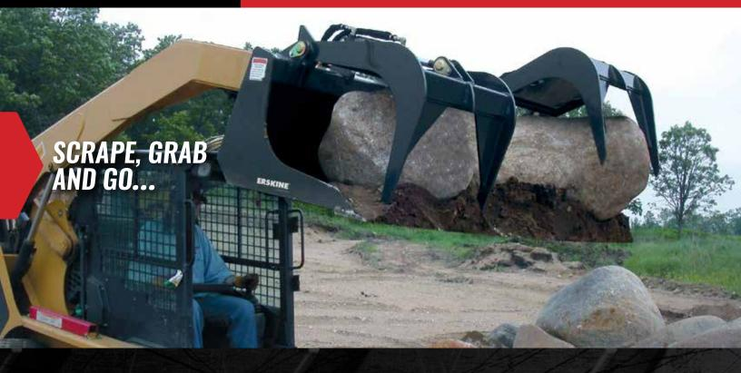
The Grapple Bucket is a wonderful tool for moving all sorts of material and earth. Sand, dirt, rocks, mud, brush, logs, there's really nothing that this grapple bucket can't move. Two independent heavy-duty grapples powered by 3,000 lb. hydraulic cylinders secure uneven and odd shaped loads. Simply a great all around attachment for almost any job.
