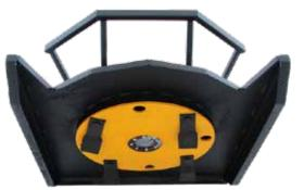
Massive, heavy-duty 450 lb. blade carrier with 3/4" steel plate. Carrier stores rotational energy to enable more power at the blade for greater cutting capacity. This design allows the blades to rotate 360° acting as a hatchet. Also features spindle seal protection reducing damage to shaft seal from wire.
