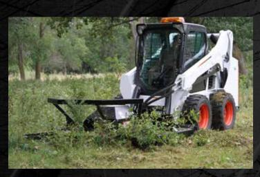
Open cut-away deck channels material to the center for most efficient cut.
