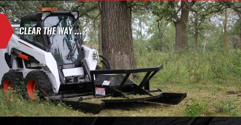
Cut, clear and mulch the heaviest brush, grass, saplings, and trees with the Heavy-Duty Direct-Drive Brush Mower. The heavy-duty, high-flow design can handle the toughest land clearing projects, and trees up to 8" diameter with your skid steer. Industrial deck is reinforced for maximum cutting potential and long-term durability. Open deck design and heavy-duty push bar make quick work of large saplings and small trees.
