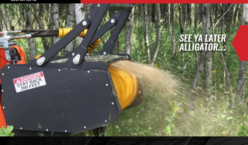
The Heavy-Duty Forestry Mulcher is a land clearing machine for breaking trails, leveling building sites, and clearing storm damage. This beast is designed with a variable displacement motor that automatically determines the best combination of speed and torque to tackle any situation.
