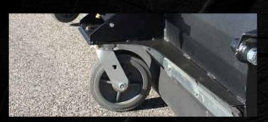
Dual heavy-duty caster wheels keep consistent pressure between the bristles and the ground
