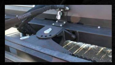
Exclusive 8° oscillating design allowing the broom head to move with the contour of the ground
