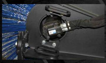
Protected direct-drive motor by Eaton Char-Lynn is mounted inside the brush arbor
