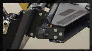
Rubber torsion system which allows the head to float up and down
