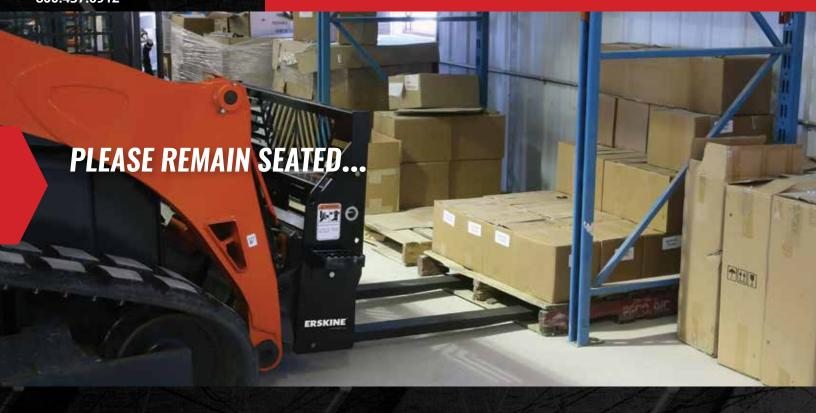
The Hydraulic Pallet Forks use hydraulic power to adjust the width between forks without leaving the operator's seat. Available with 48" or 60" forks with load ratings of 5,500 lb. at 24".
