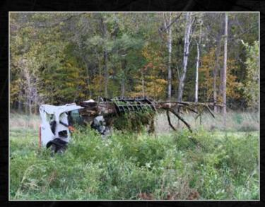
Gathers and piles brush as well as limbs and logs. Our unique design allows for vertical pick-up and dumping of debris.
