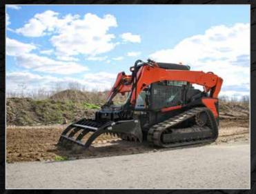
Use rake for gathering... or sink teeth in the ground for digging out roots or rock.
