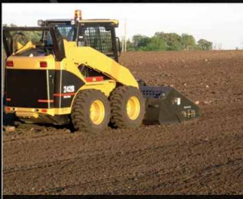
The Landscape Rake also breaks up lumpy soil, while grading, leveling, scarifying - preparing the soil in a one-step process.
