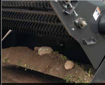
12 reversible bolt-on rake bars manufactured from 7 gauge steel.
