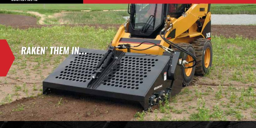
An attachment that pays for itself in a very short amount of time, replacing your hand labor work crew. The Landscape Rake was designed to remove small to medium-sized rock as small as 3/4" along with unwanted roots and debris. The Landscape Rake also breaks up lumpy soil, while grading, leveling, scarifying – preparing the soil in a one-step process. This is the perfect tool for preparing a seedbed, sodding or lawn leveling.
