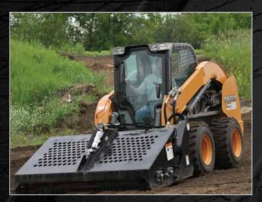
The Landscape Rake was designed to remove small to medium-sized rock as small as 3/4" along with unwanted roots and debris.
