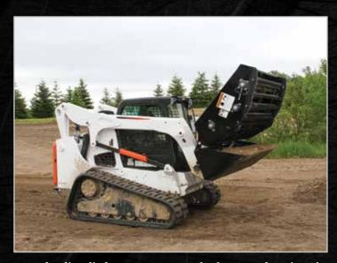
Hydraulic cylinder opens top cover for fast, easy dumping of the large containment bucket.
