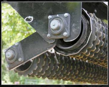
Front rollers crush lumps, press down small stones, and form a firm seed bed. Rear rollers split the shallow ridges formed by front rollers.
