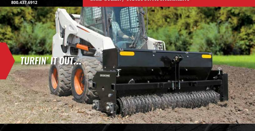
The Landscape Seeder is built to handle all turf and landscape seeds. Grass seed is a very expensive commodity. Notched rollers properly place the grass seed in the top 1/2" of a properly prepared seedbed, resulting in maximum seed germination. Seedbed is left smooth and firm with small stones pressed down. Because of this precision placement seeding rates can be reduced up to half of the rates previously used.
