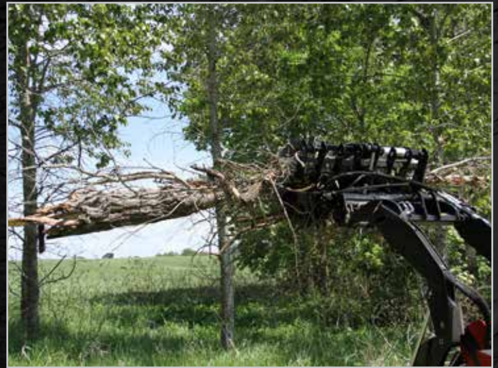
Optimal spacing between teeth allows unwanted debris to fall through.
