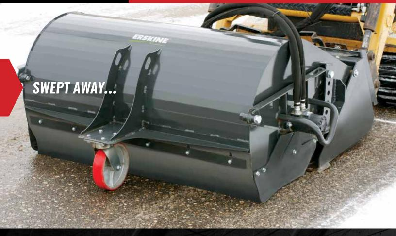
Sweep clean and scrape mud going forward or in reverse. Ideal for construction, industrial or municipal jobs, the Mini Pick-Up Broom is easy to attach and simple to operate. Replaceable cutting edge helps remove caked-on mud, while the sweeper's poly bristles deposit dirt and debris in the container, which can be dumped when full.
