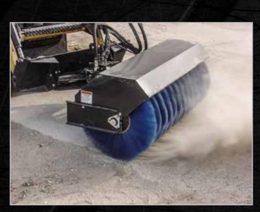
The direct drive motor turns the broom that angles 25° in both manual and hydraulic configurations.
