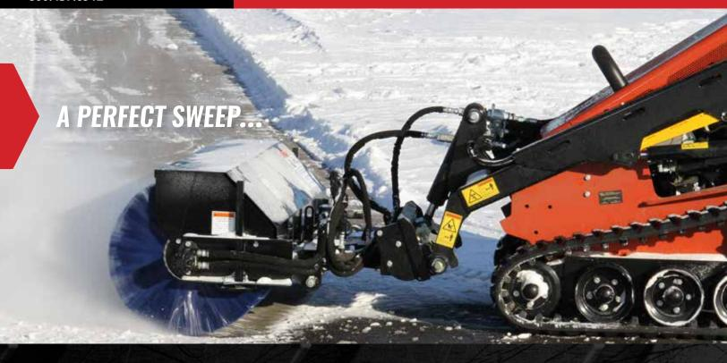
The Mini Power Angle Broom is designed for heavy-duty sweeping of dirt, snow, and other unwanted material. It quickly mounts to your mini skid steer. Featuring a 48" width and optional hydraulic angle change, this attachment is designed to go anywhere to get the job done!
