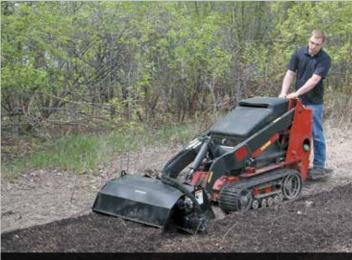
Bi-Directional rotation increases efficiency by saving time and labor.
