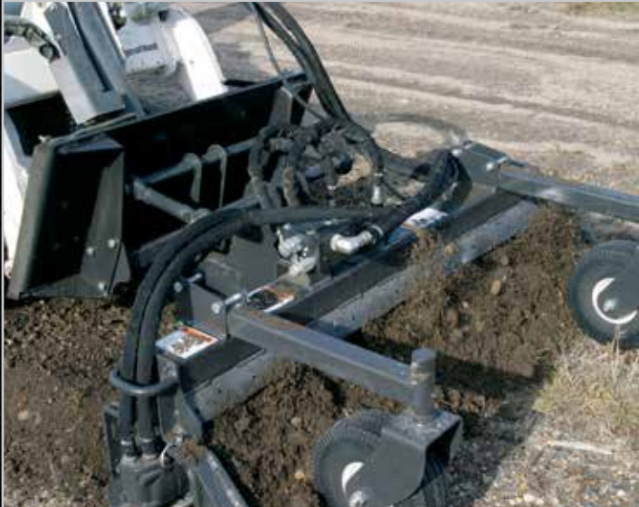
Floating mounting system follows the contour of the ground.
