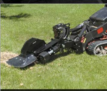
Offset cutting wheel allows the operator great visibility.
