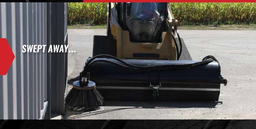
Sweep clean, scrape mud going forward or in reverse. Ideal for construction, industrial or municipal jobs, the Pick-Up Broom is easy to attach and simple to operate on your skid steer. The reversible cutting edge helps cut loose caked-on mud, while the sweeper's poly bristles deposit dirt and debris in the container which can be dumped when full.
