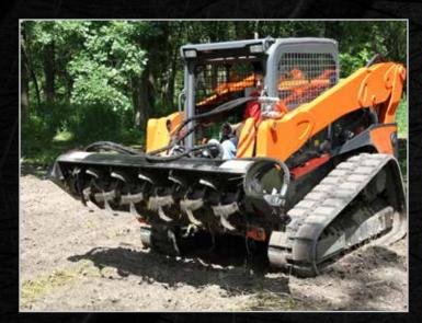
Tines are designed to allow "flex" so damage is less likely when a large rock is impacted and turned over through the tines.
