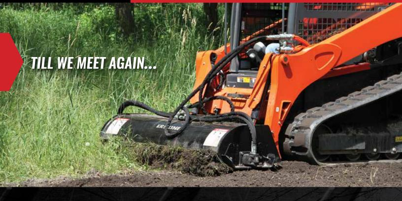
This is a perfect tool for preparing gardens, food plots or seedbeds. The bidirectional rotation saves time and labor as it allows you to quickly pulverize soil and cover your tracks. The dual direct-drive motors and replaceable, double-edge hardened tines keep you in the fields working, not in the repair shop.
