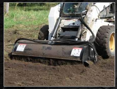
Dual direct-drive motors give high production with lower maintenance
