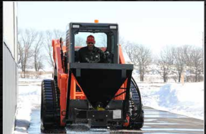
Sidewalk Kit featured above. AR400 agitator and AR400 cutting edge.
