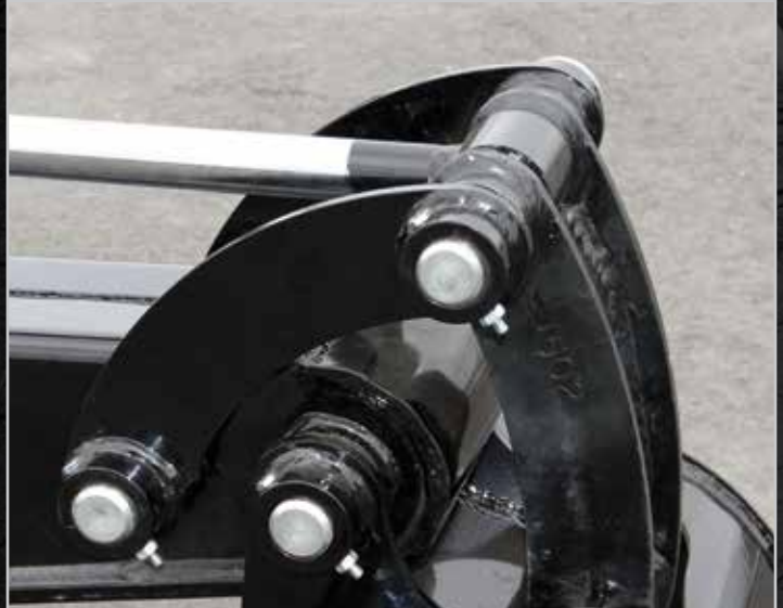
Greaseable pin points for easy maintenance.
