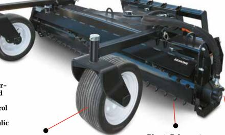
Large solid rubber tires allow easier maneuverability over rough terrain Direct-Drive motor gives higher production with lower maintenance Optional:
