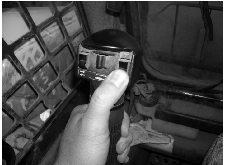
PUSH AND HOLD TO ENERGIZE DIVERTER
