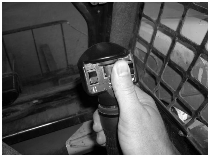
OPERATE AUXILIARY HYDRAULICS TO TILT
