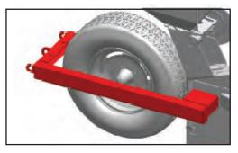
3. Bolt on tire scraper such that there is no more than 3/16" clearance between tire and scraper
