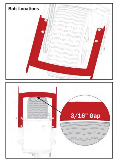
2. Adjust draw bar such that there is no more than 3/16 clearance between tire and scraper
