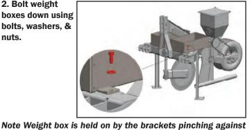
the frame. Once concrete is added, the box will be solidified.
