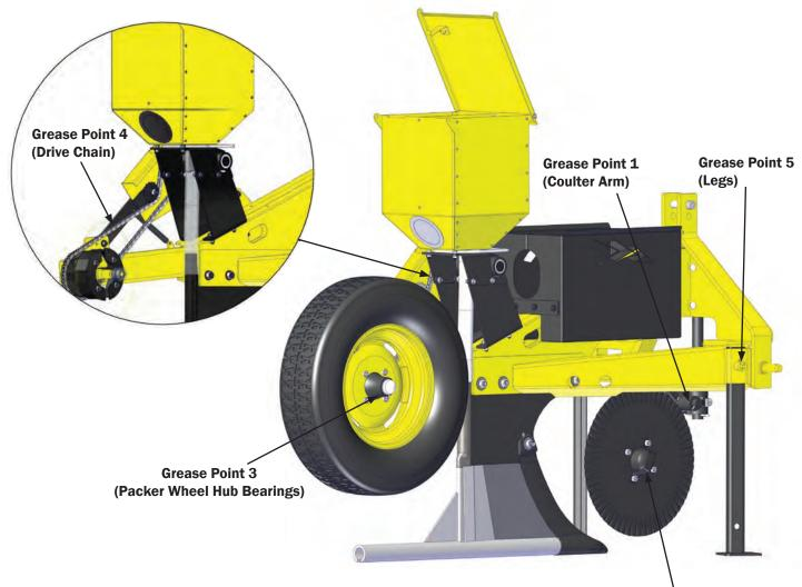
Grease Zerk Point 2 (Back of Coulter Hub)
