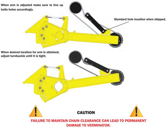
Remove links as necessary. To maintain proper spacing between chain. We provide 7 quick links already attached to chain. Reduce or add as needed to obtain proper chain clearance.
