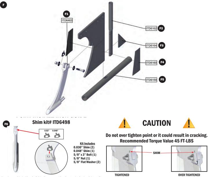
Use the provided shims individually or a combination to obtain the tightest fit between the point and the shear.
