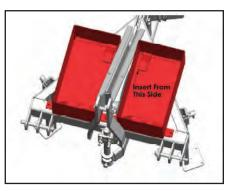
2. Bolt weight boxes down using bolts, washers, & nuts.
