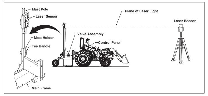
Figure 19. Components of the Automatic Control System
