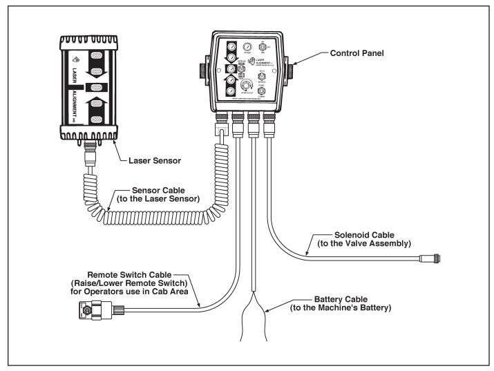
Figure 16. Single Automatic Control System
