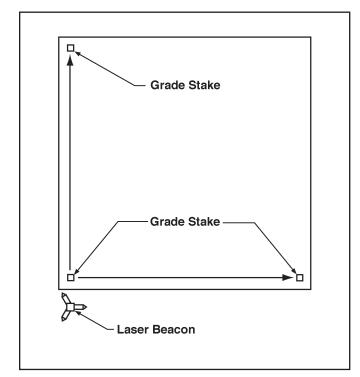
Figure 23. Method Two: Align Rotating Laser with Grade Stakes
