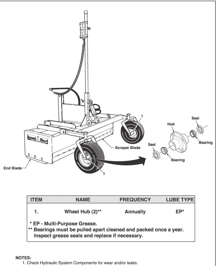
2. Check and tighten all bolts and nuts for scraper blade and end blades, weekly.
