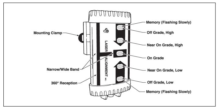
Figure 12. Laser Sensor Features
