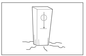
Figure 22. Grade Stake with Elevation Mark
