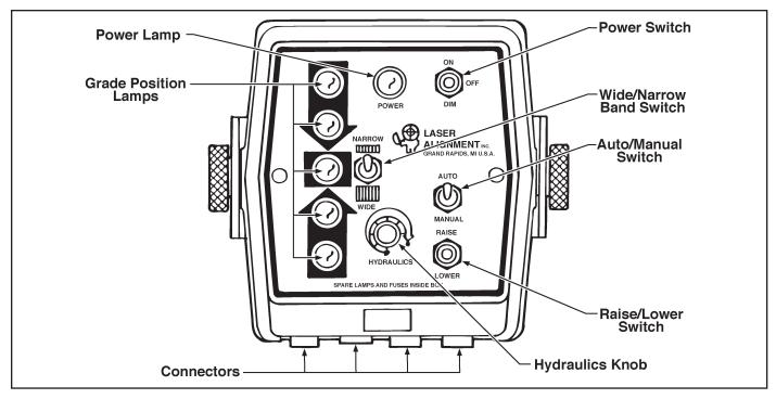
Figure 2. Control Panel Features
