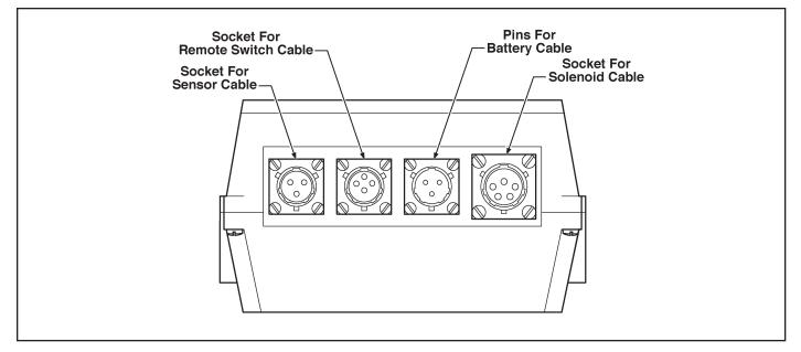
Figure 17. Bottom View of Control Panel
