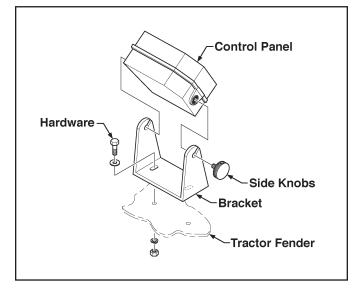
Figure 18. Control Panel Mounting
