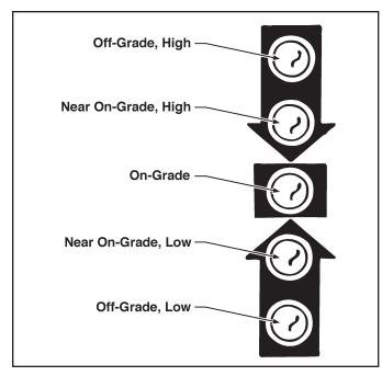
Figure 5. Grade Position Lamps
