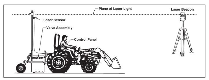
Figure 1. Plane of Laser Light with Components of the Automatic Control System
