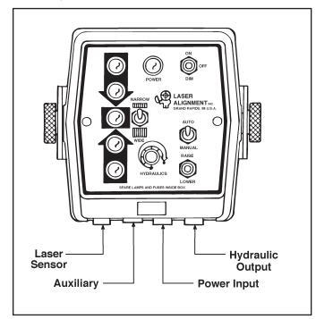
Figure 10. Cable Connectors
