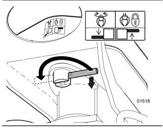
Fig. 15-Grapple Pivot Lock Lever
