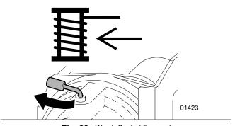
Fig. 22-Winch Control Engaged
