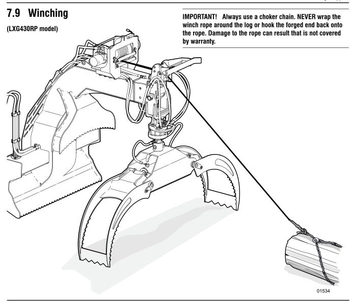
Fig. 34-Winching Logs
