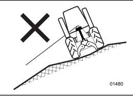
Fig. 5—Never Winch from the Side on a Slope
