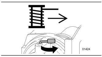
Fig. 21 – Winch Control Disengaged (Freespool)
