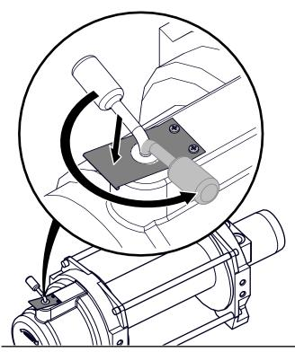
Fig. 32 - Winch Disengaged (Freespool)
