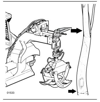
Fig. 30 - Using Grapple Push Bar
