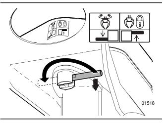
Fig. 28 - Grapple Pivot Lock Lever
