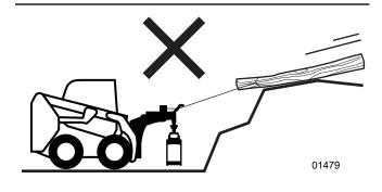
Fig. 6-Never Winch Down Slope
