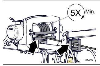
**Fig. 31 –** Winch rope must pass through guides. Leave minimum five wraps on drum.
