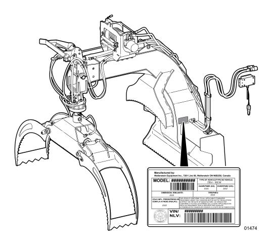
Fig. 1 – Serial Number Plate Location (Typical)
