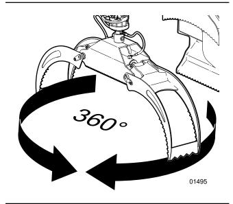
Fig. 16-Hydraulic Rotator
