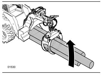
Fig. 26-Parallel Lift with Cantilever
