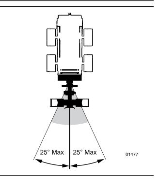
Fig. 3-Safe Winch Angle
