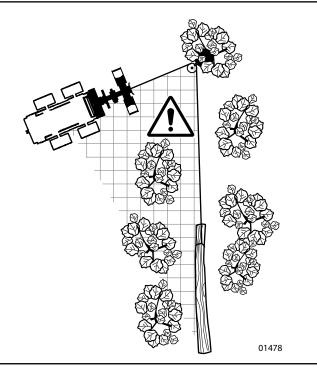
Fig. 4-Using a Snatch Block or Self-releasing Pulley
